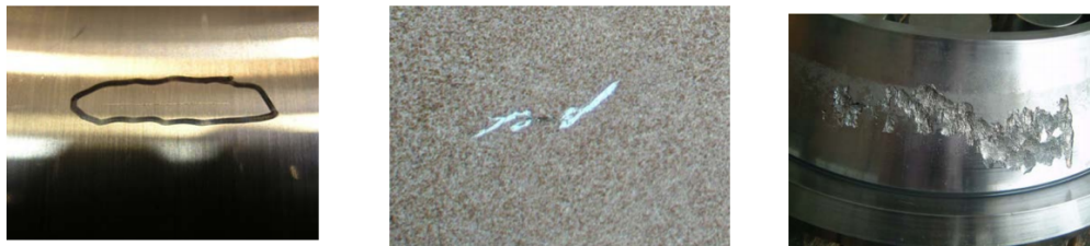
Figure 2.11: Axial cracks dominated by high-speed and intermediate-speed stage bearings inner raceway [37].
