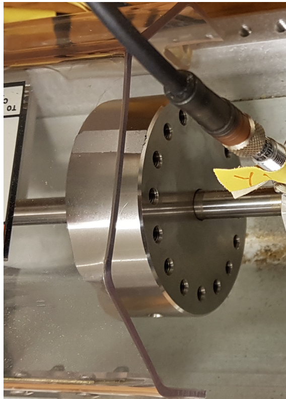
Figure 5.7: The attachment-placement of weights to produce fault cases.
