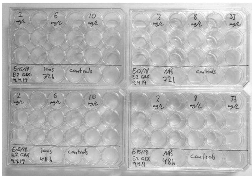
Figure 9: Test setup for GRX. Two sets of plates were prepared, one for analysis at t=48 h and one at t=72 h.
