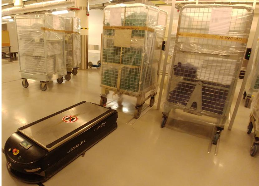
Figure 7: An AGV about to pick up a hamper
