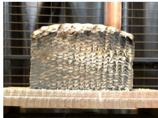
Figure 3.8: Weld beads from the front view
