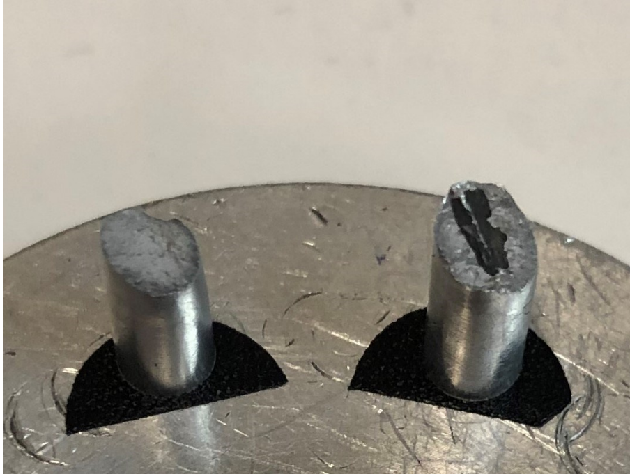
Figure 4.5: Fracture surfaces of the permanent mold cast tensile specimens P11 (left) and P8 (right). Sliced from tensile test specimens and glued to the fixture plate for SEM. The black area in P8 (right) is pollution and oxide film.
