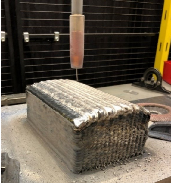
Figure 3.7: Part deposited by WAAM. Rectangular block
