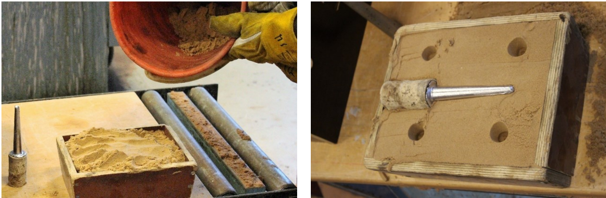
Figure 3.6: Forming the sand mold, with impression of a permanent mold casting
