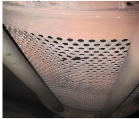
(b) One of the perforated plates with blown out section.
