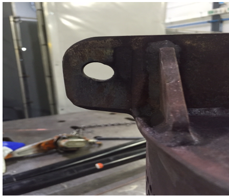
(c) Oval Bolt holes found in the diffusor.
