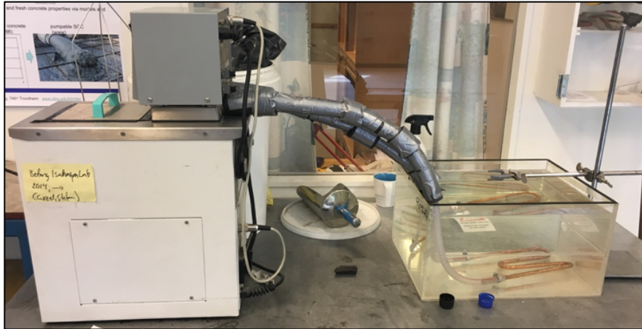
Figure 10 The set up for Julabo and water bath
