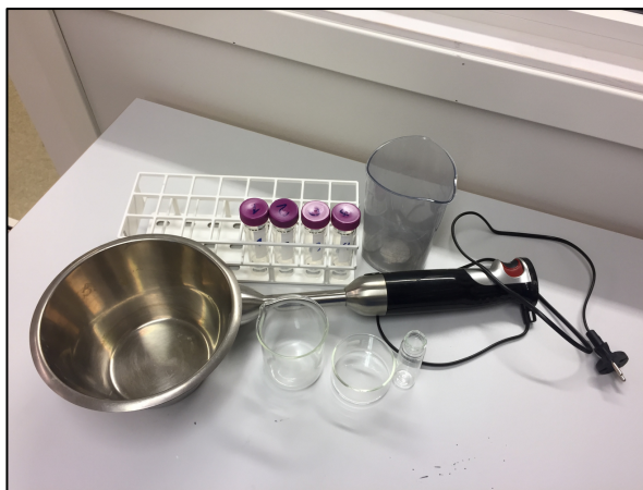
Figure 6 The equipment: a metal bowl for dry particles, falcon tubes, a beaker glass, a cup, a glass bottle and the hand blender with its steel blade and plastic container.
