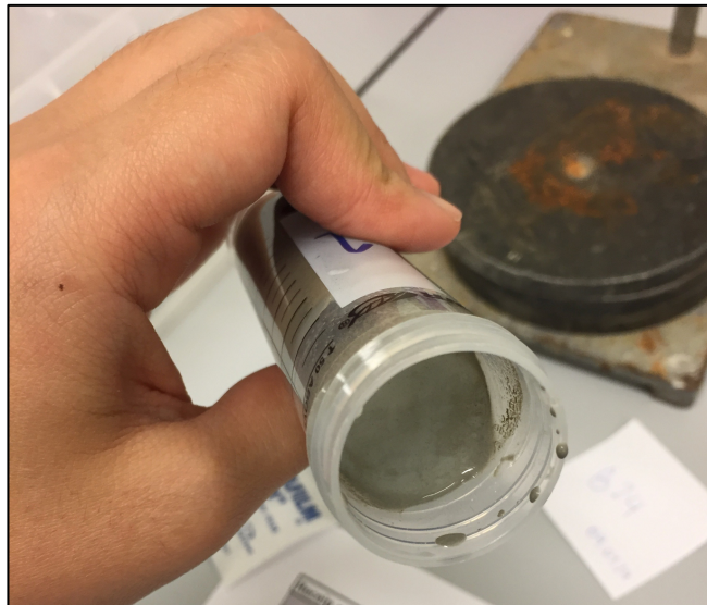
Figure 11 The unpacked paste after centrifugation from mix no. B24
