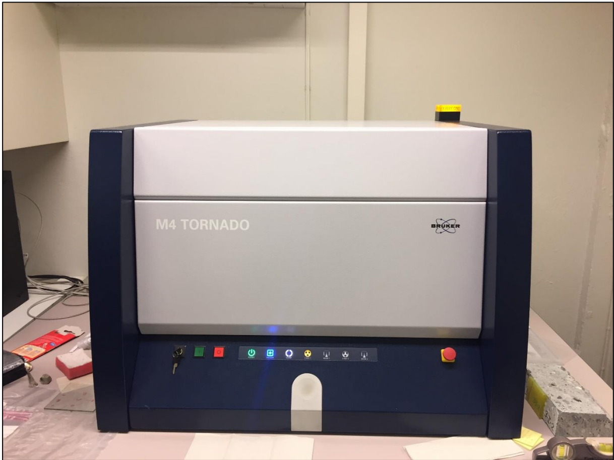
Figure 4-8: Illustration of the \mu -XRF machine used. [Vådahl, 2019]
