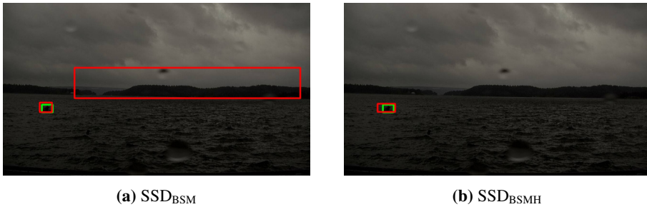
Figure 6.4: SSD B SM detects land as boat. Red bounding boxes are boat detections, green bounding boxes are ground truth.
