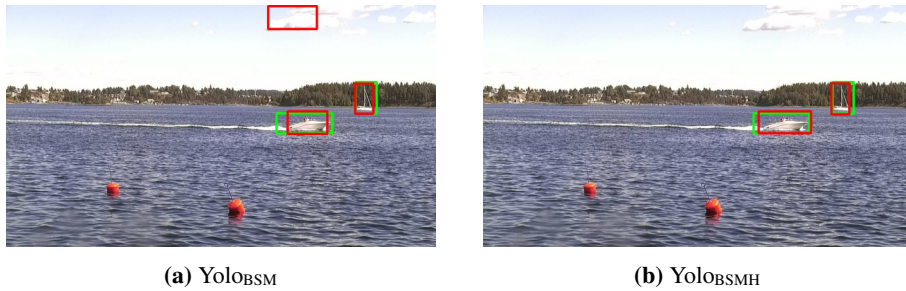
Figure 6.6: Yolo BSM misclassifies a cloud as a boat, Yolo BSMH does not. Red bounding boxes are detections, green bounding boxes are ground truth.
