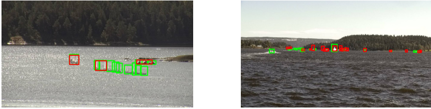
Figure 7.1: Yolo BSMH on cluttered small boats, red bounding boxes are detections, green bounding boxes are ground truth.
