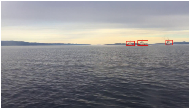
Figure 3.1: Detected boats by Yolov3 on image from Trondheimsfjorden.
