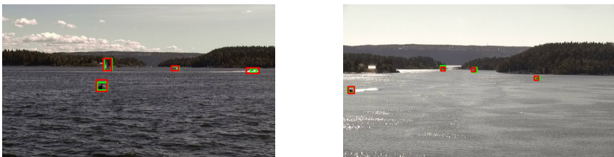
Figure 7.2: Yolo BSMH on separated boats in BoatsClose BoatsFar, red bounding boxes are detections, green bounding boxes are ground truth.
