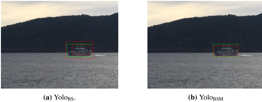
Figure 6.16: Example of Yolo BS detecting same boat twice.
