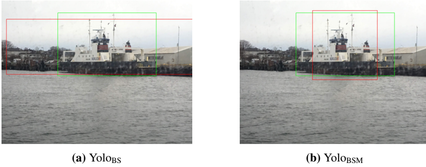
Figure 6.15: Example of Yolo BS over estimating size of ship.
