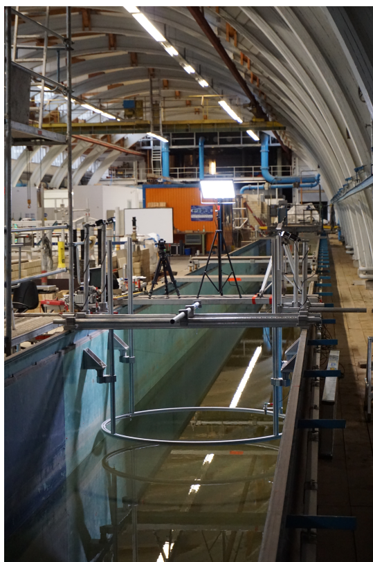
Figure A.2: Picture of the ring for attaching the soft-mooring system
