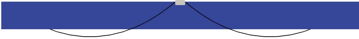
Figure 5.4: Initial position of the floating barge and the mooring ropes of a slack configuration
