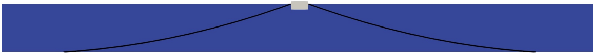
Figure 5.5: Initial position of the floating barge and the mooring lines of a taut configuration
