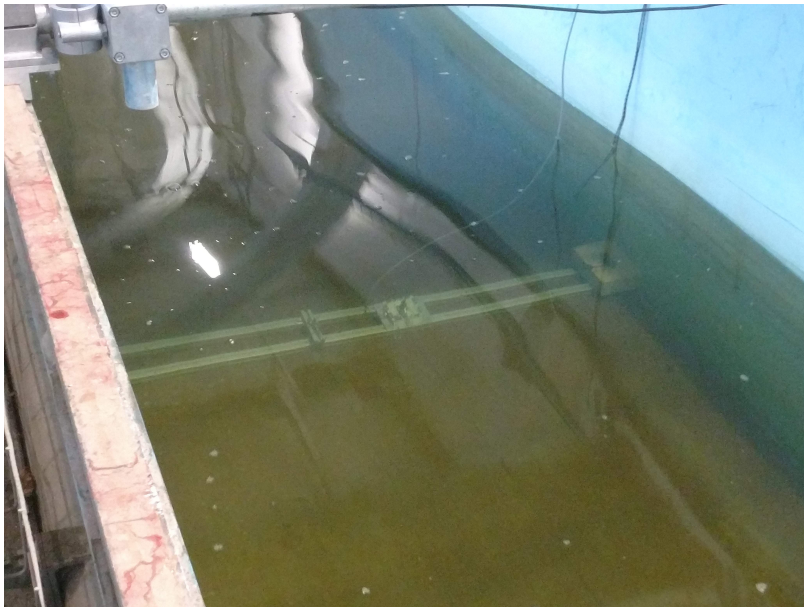
Figure A.5: The weight-ballasted attachment points on the floor
