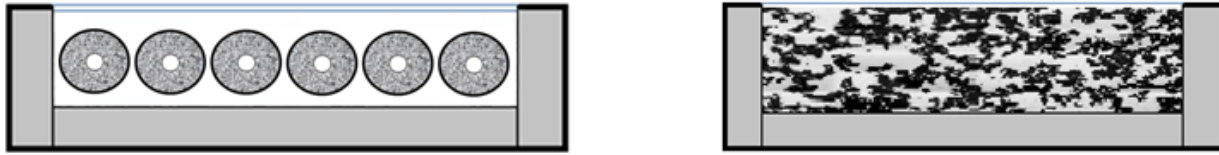
Figure 6.9: Possible tubular and rectangular adsorption bed
