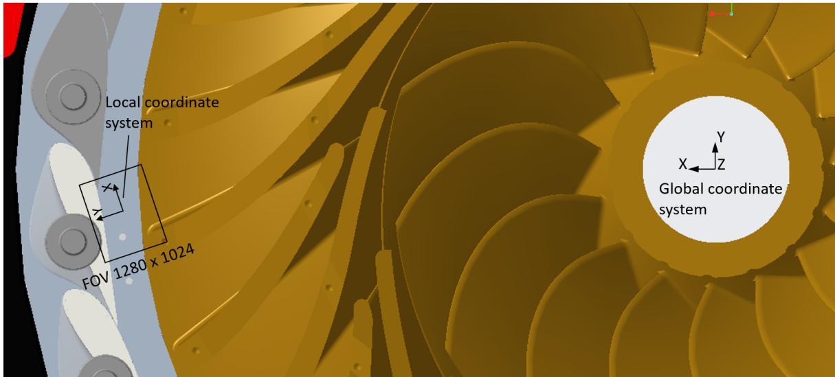
Figure A.1: An overview of the local coordinate system of the FOV and the global coordinate system of the turbine.
