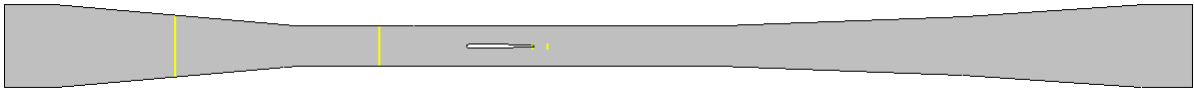
Figure 3.16: Location of the sampling lines (in yellow) for the velocity profiles in the inlet location dependence study. The locations are z = 0.630 m, z = 1.381 m, z = 1.943 m and z = 1.99952 m ( 9.9D m downstream of trailing edge) downstream of the original inlet location along the centerline.
