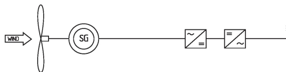
Figure 2.6: The offshore direct drivetrain configuration with full converter used in this thesis (Hau and von Renouard, 2003)
