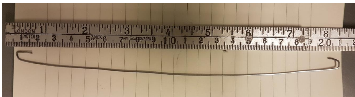
Figure 18: The Mo-wire made for the melting experiments
