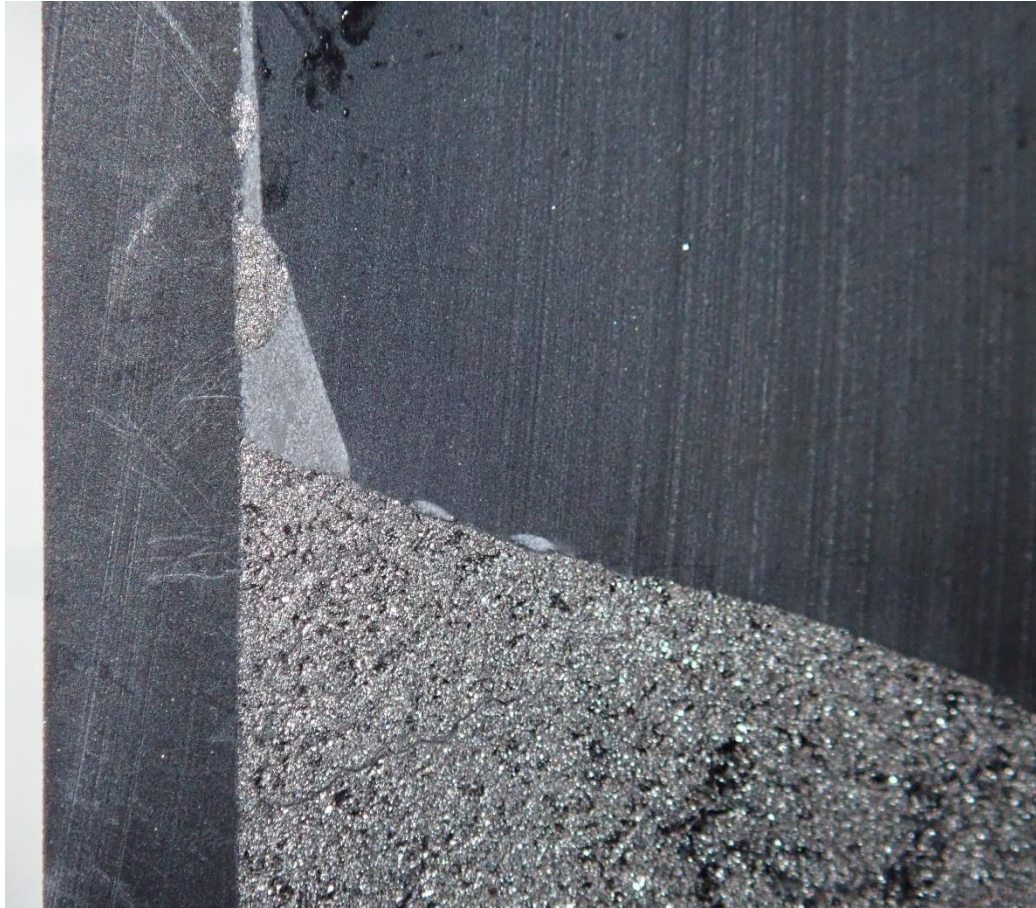
Figure 24: Top corner of sample from experiment 3, showing an example of metal and slag creeping up the crucible wall, indicating good wetting
