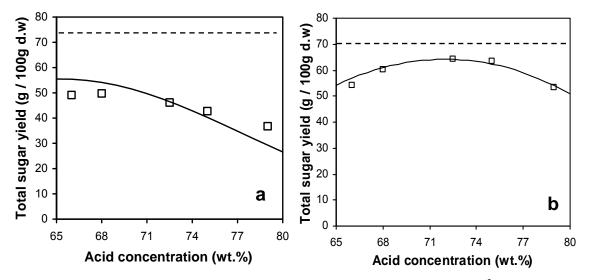
**Fig. 4.** Validation of the total sugar yields dependency on acid concentration at 35°C and 60 minutes. Experimental (□) versus predicted (—), Theoretical maximum (----) (a) aspen (b) pine
