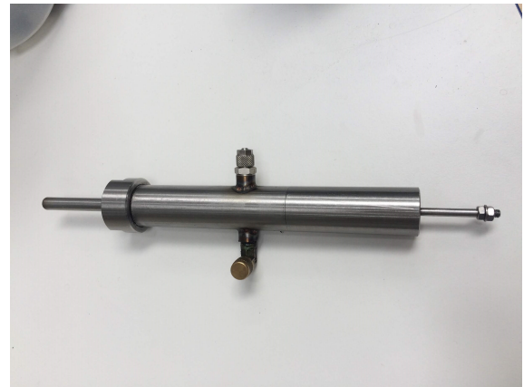
(b) The cylinder including two pistons and a flushing mechanism
