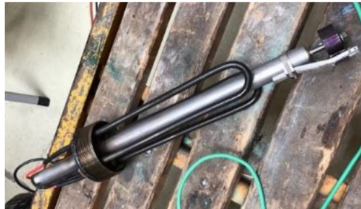
Figure 50: The heating module consisting of the bimetallic spring and the heating elements attached to the plug
