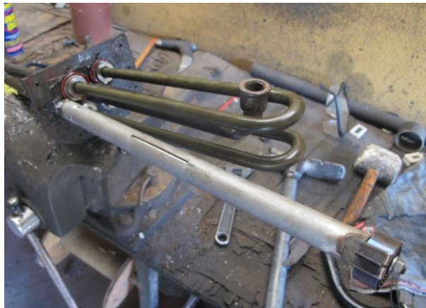
Figure 20: The bimetalllic spring connected to the heating element attachment
