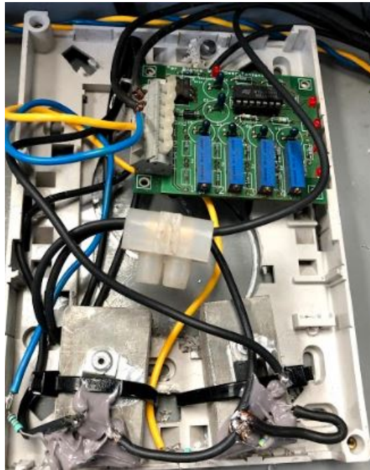
Figure 29: The actual controller box. The controller board at the upper part and the two switches with the connected resistors and aluminum below
