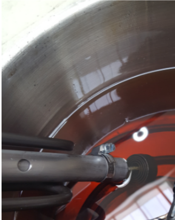
Figure 52: The bimetallic spring submerged in oil during testing
