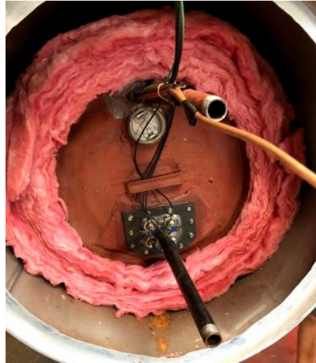
Figure 13: The storage tank. Lower: the heating elements and the outlet. Upper: pipes from the coil, thermal sensor (green cable) and the inlet
