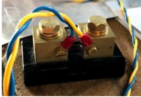
Figure 7: The shunt used to measure the voltage
