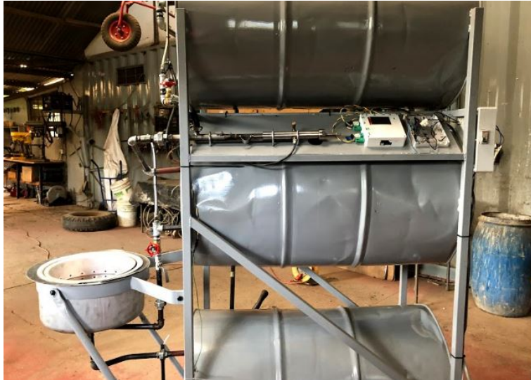
Figure 17: The system after connecting the cooker, the pistons and plumbing
