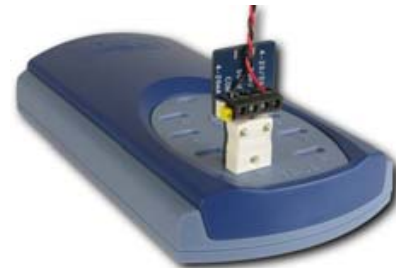
Figure 2: The terminal board fitted to the USB TC-08
