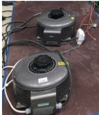
Figure 57: Adjustable voltage sources, rated 20 A, used for testing the spring
