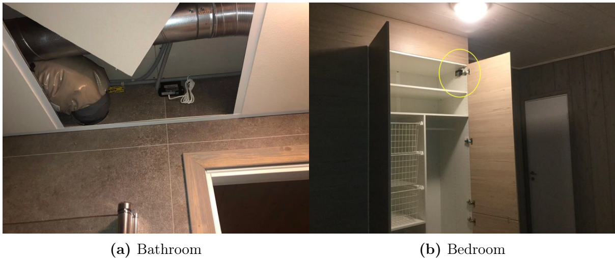
Figure 3.6: Placement of the internal climate sensors (Kvande, T., Gullbrekken, L., and Geving, S., 2018)
