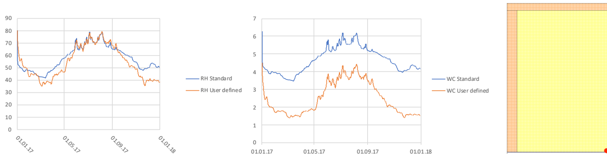
Figure A.2: RH and moisture content of the mineral wool close to the SVB
