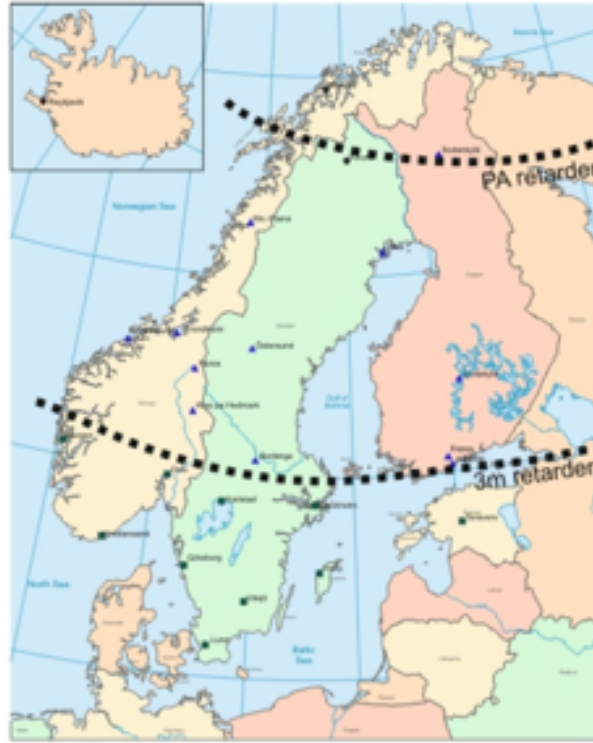
Figure 1.7: Geographical limits of the use of a vapour retarder, s_d = 0, 1 - 4, 4 , and vapour barrier s_d = 3m (Bludau, C. and Künzel, H. M., 2009)
