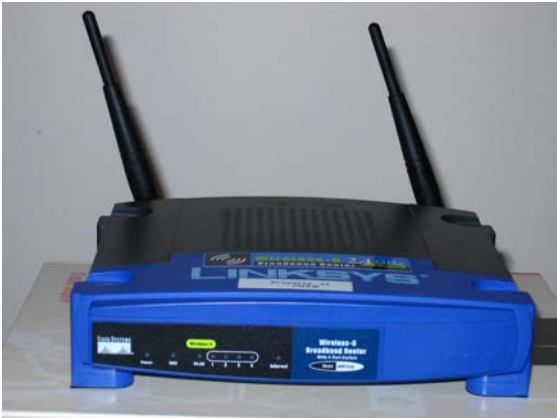
Figure 37 The orientation of the antenna from a front view showing the 110-degree angle used. Where 90 degrees indicates that the antenna's are vertical.
