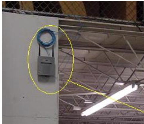
Figure 5-2 Access Point Installed on a Wall
