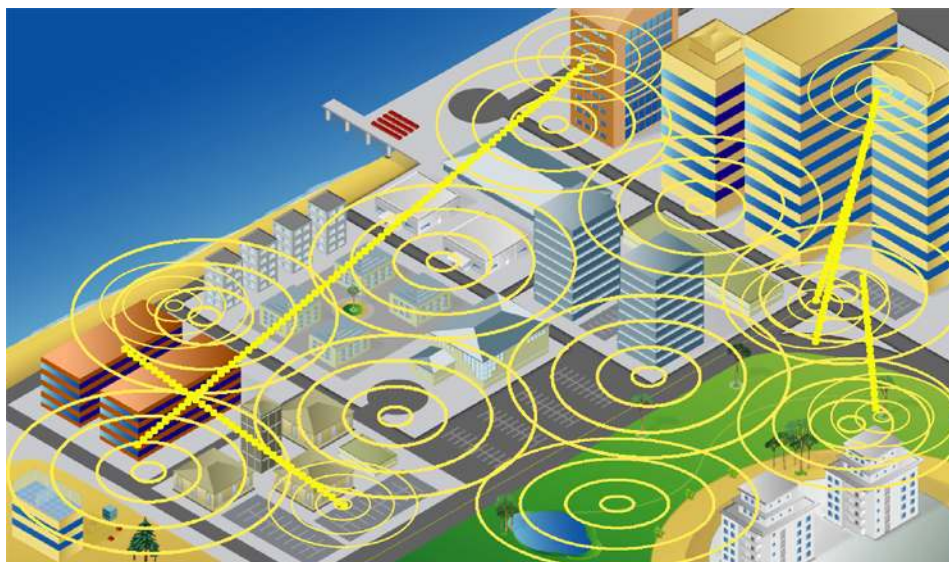
Figure 1. Two-level Wireless Infrastructure: Rooftop, Power Poles, and Street Lights
