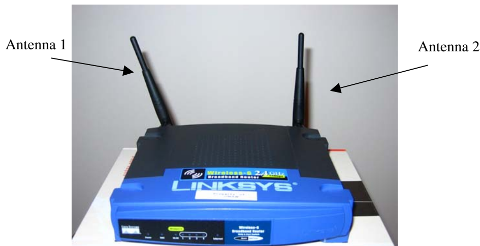
Figure 38 The orientation of the antenna from a front view showing antenna 1 at 110 and antenna 2 at 90 degrees
