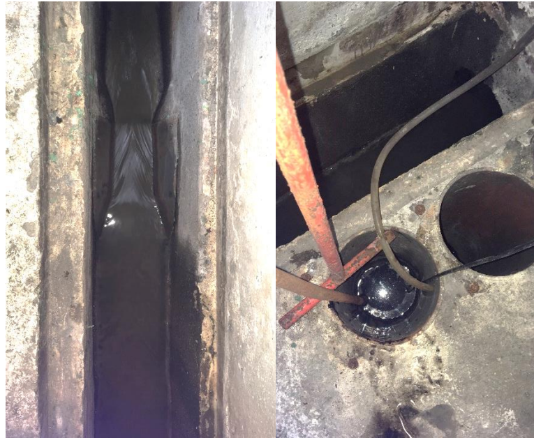
Figure 4.9. Left: Flow through the Palmer-Bowlus flume. Right: the cylinder with the measuring sensor (Photo Birgitte Taugbøl Kragset)
