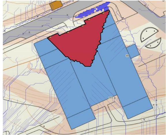
Figure 6.5 (Left) Watershed contributing runoff to the storm drains located in the northern area.
