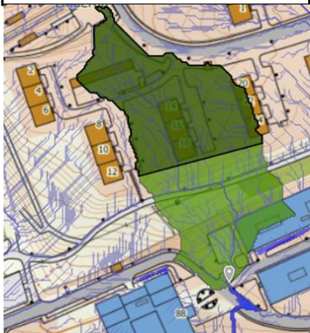
Figure 6.11 Privately drained area as seen in SCALGO.
