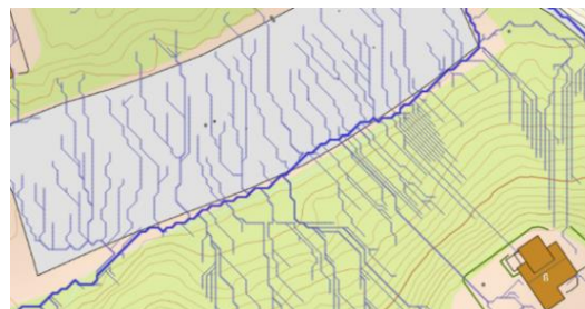
Figure 4.1 Example of the flow accumulation tool in SCALGO.
