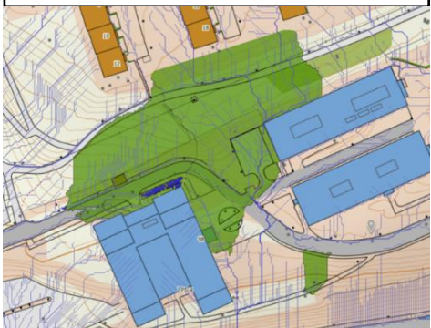
Figure 6.18 Total runoff contributing area marked in green.
