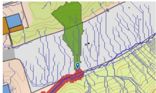
Figure 4.3 Example of depression-free flow in SCALGO.
