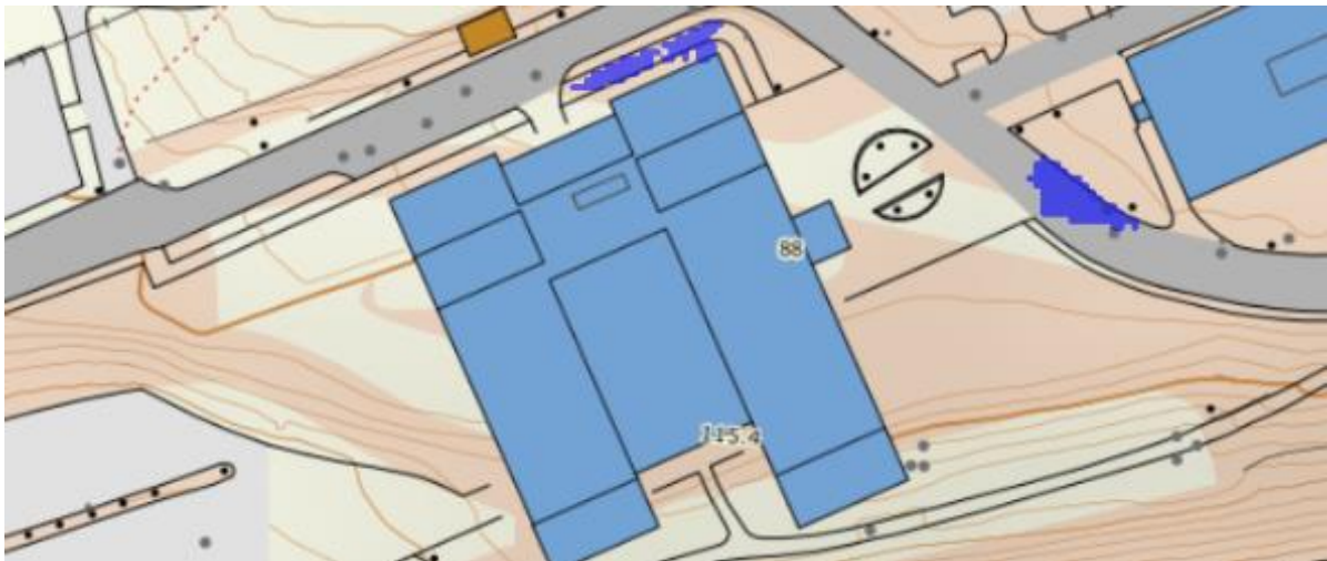
Figure 6.9 The two buildings that contribute runoff to the Siemens detention system. The main building in the centre of the map (blue) has an area of approximately 2970\text{ m}^2 , and the small orange building north of the main building has an area of approximately 32\text{ m}^2 .
