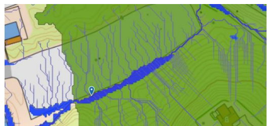
Figure 4.5 Example of flash-flood mapping with a water depth of 6 mm in SCALGO.
