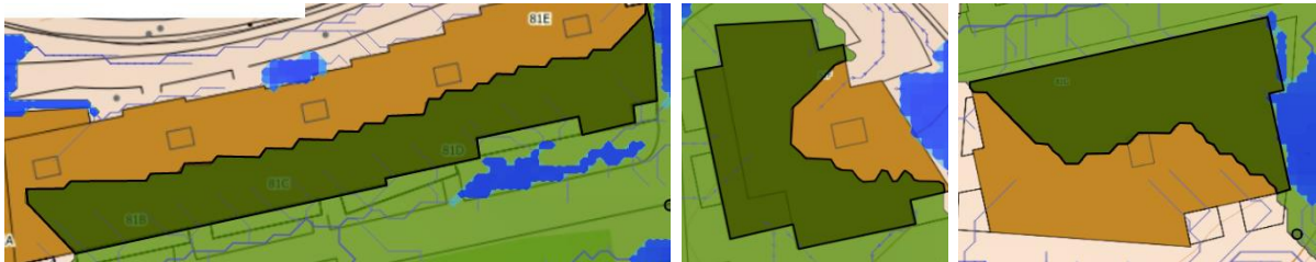
Figure 5.8 Identification of rooftop area included in the watersheds connected to the open drain on the South-Eastern area. Rooftop 1 (top) has a green area of 592\text{ m}^2 , rooftop 2 (left) has a green area of 230\text{ m}^2 and rooftop 3 (right) has a green area of 272\text{ m}^2 .
