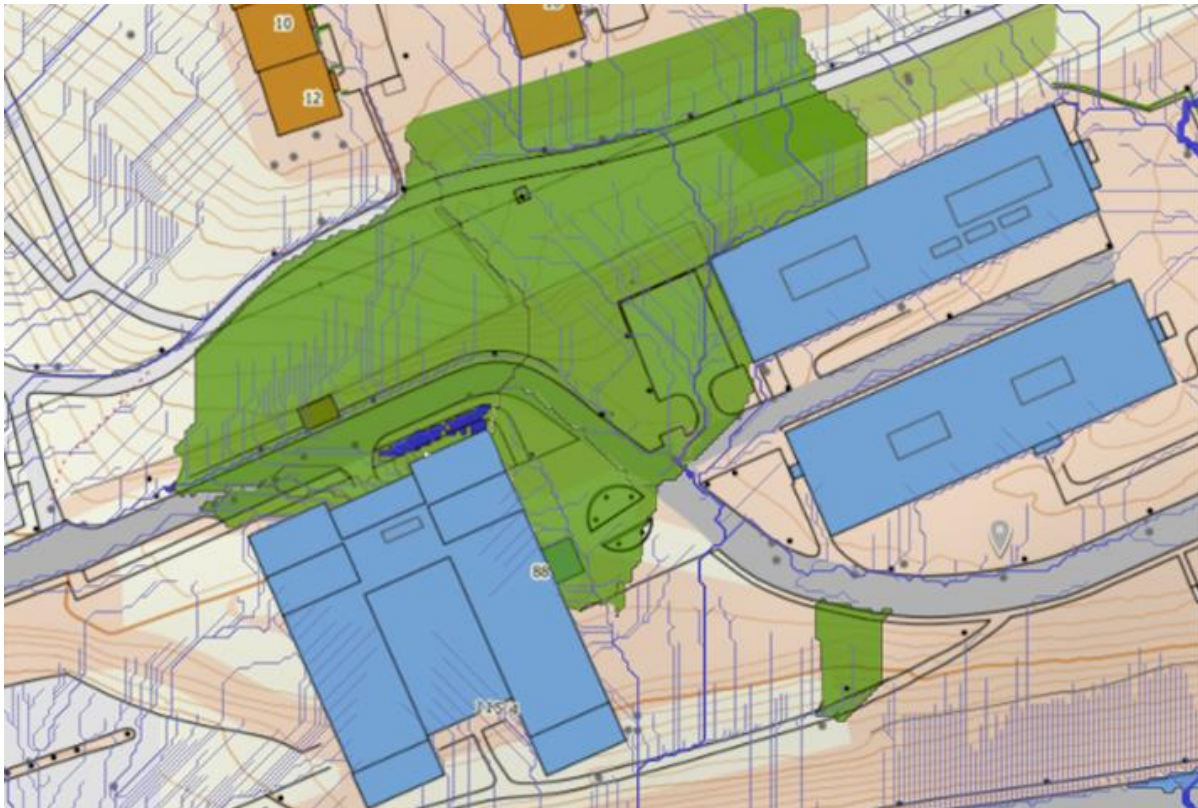
Figure 6.19 Final runoff contributing area marked in green. The runoff area also includes the main building in the lower left part of the figure.
