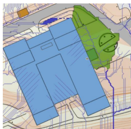
Figure 6.7 (Left) Watershed contributing runoff to the storm drain located in the central area.
