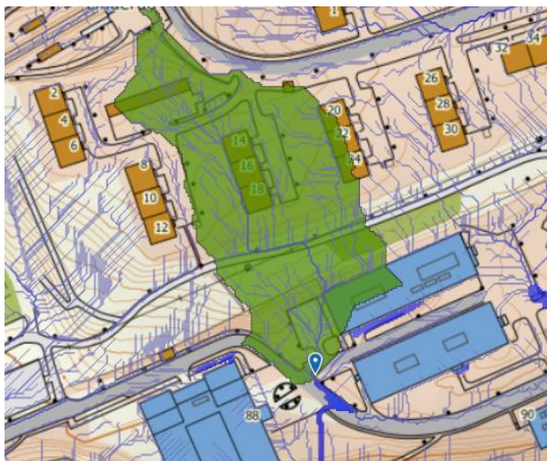
Figure 6.3 (Left) Area contributing runoff to the purple storm drains according to SCALGO.
