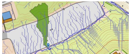
Figure 4.4 Example of flash-flood mapping with a water depth of 0 mm in SCALGO.
