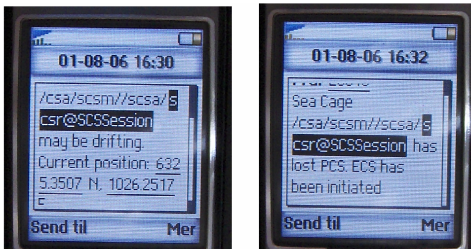
Figure 9-12: The SMS-warnings generated for GPS-position deviation (left) and link failure (right)
