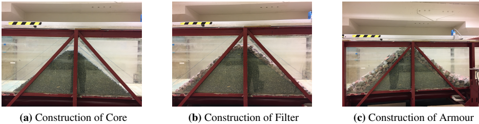
Figure 4.5: Construction of Breakwater Model Step-by-Step
