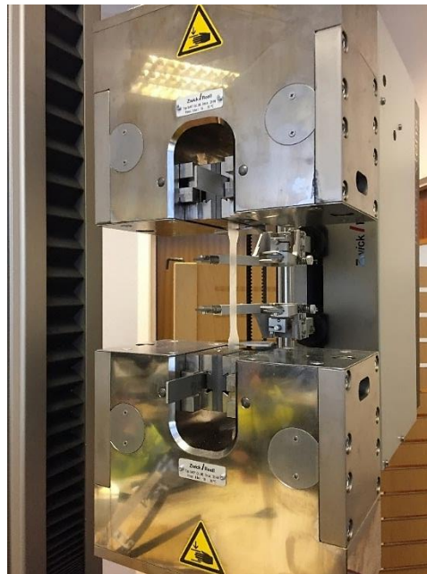
Figure 3.3: Picture of the tensile test machine in the Metallurgical Laboratory in Holmestrand.
