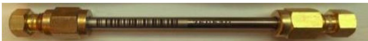
*Figure 11. Sorbent tubes with couplings.*
