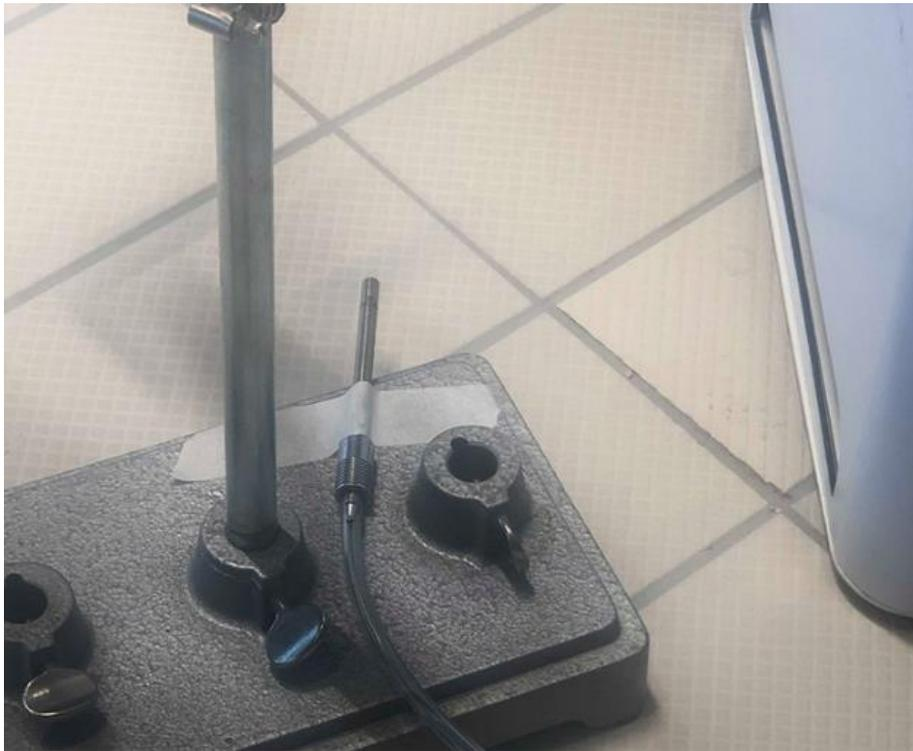
*Figure 15. Sorbent tube samples filtered air.*
