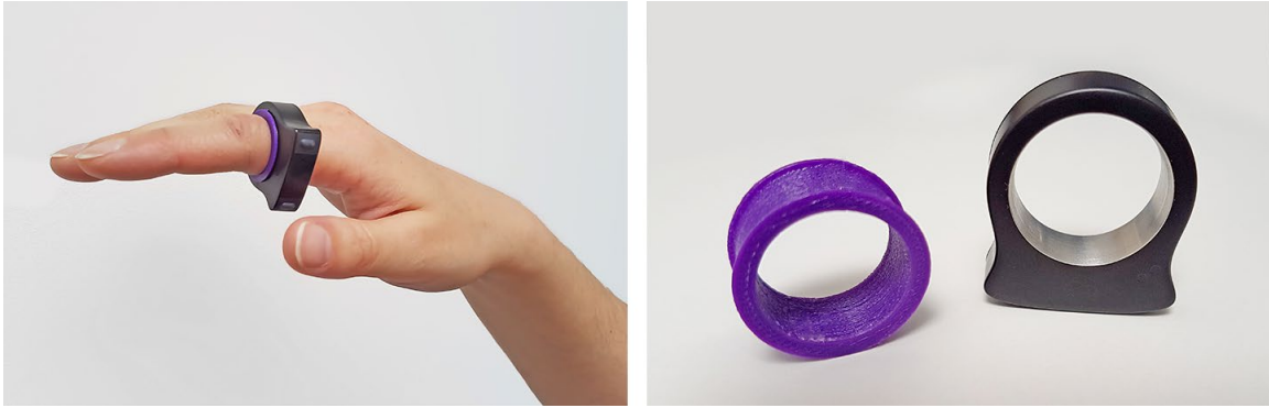
Figure 3. Nod gesture ring with thumb-facing touch-area / 3D-printed flexible adapter
