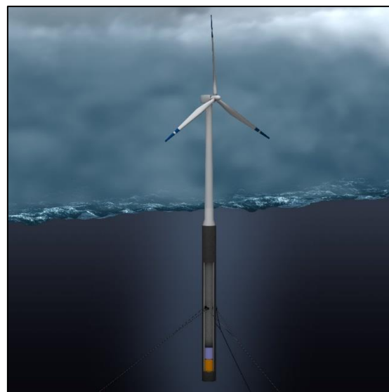
Figure 2:2 Spar buoy design proposed by Equinor (9)
