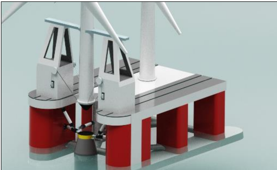
Figure 5.3: OWT hanging in initial position.
