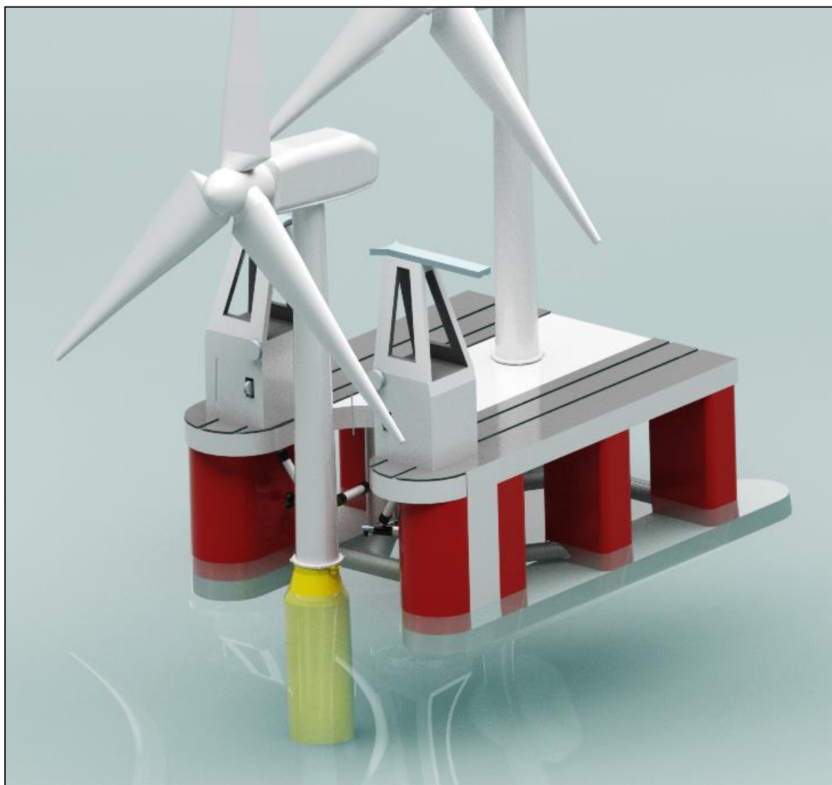
Figure 5.5: OWT is released from the installation vessel and attached to the spar.
