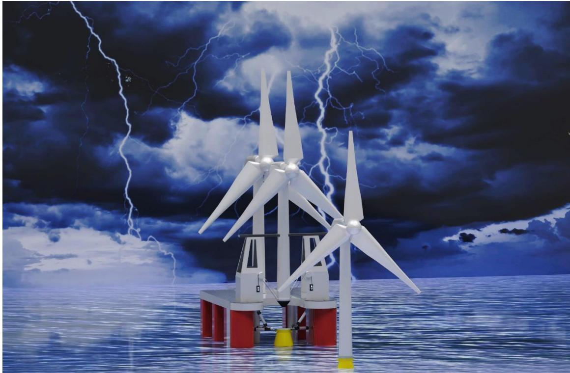
Figure 4.8: Illustration of the installation vessel with pre-assembled OWT's in action.
