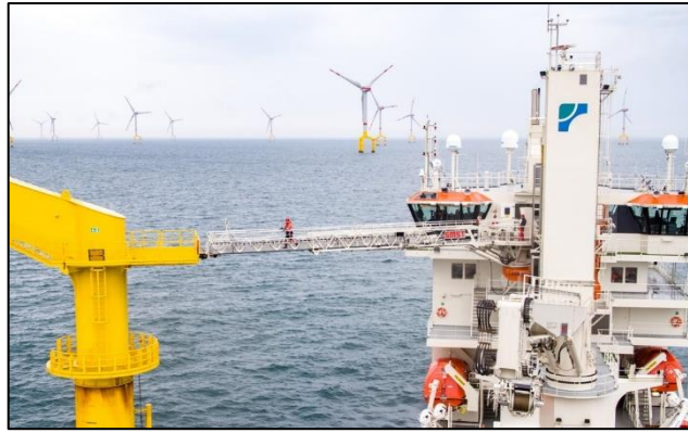
Figure 2.2: Illustration: Motion compensated gangway for safe transfer from vessel to platform.
