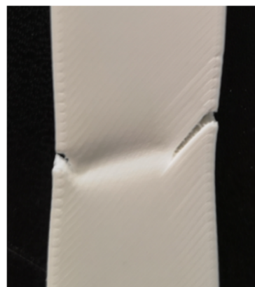
Figure 4.2: Diagonal fracture along pattern
