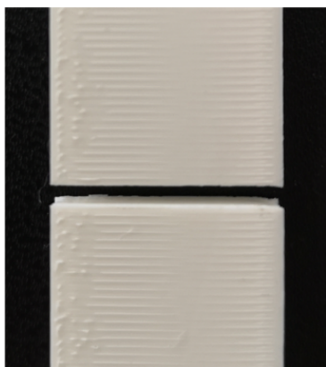
Figure 4.1: Clean fracture along pattern
