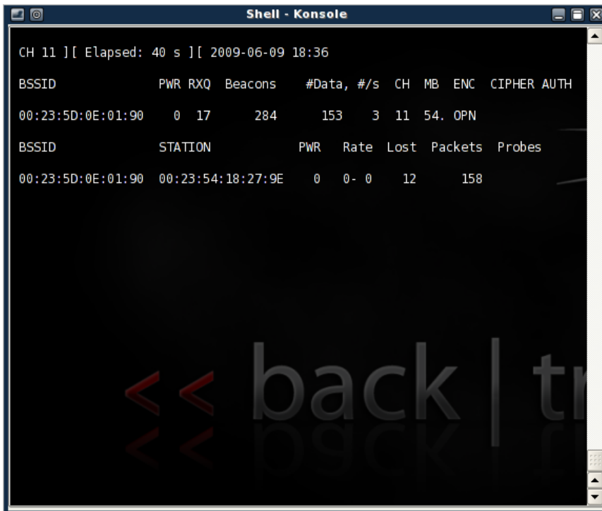
Figure 3.3: Screenshot from airodump displaying traffic on the Wireless Trondheim access point and an associated client
