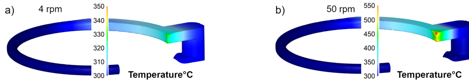
Figure 11. Temperature level in the extrusion grip zone. (a) rotational speed 4 RPM; (b) rotational speed 50 RPM.
