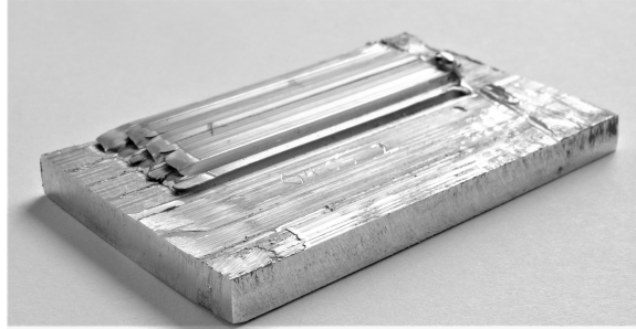
Figure 6: Photograph of a two-layered sample of AA6082 (4 + 3 stringers).
