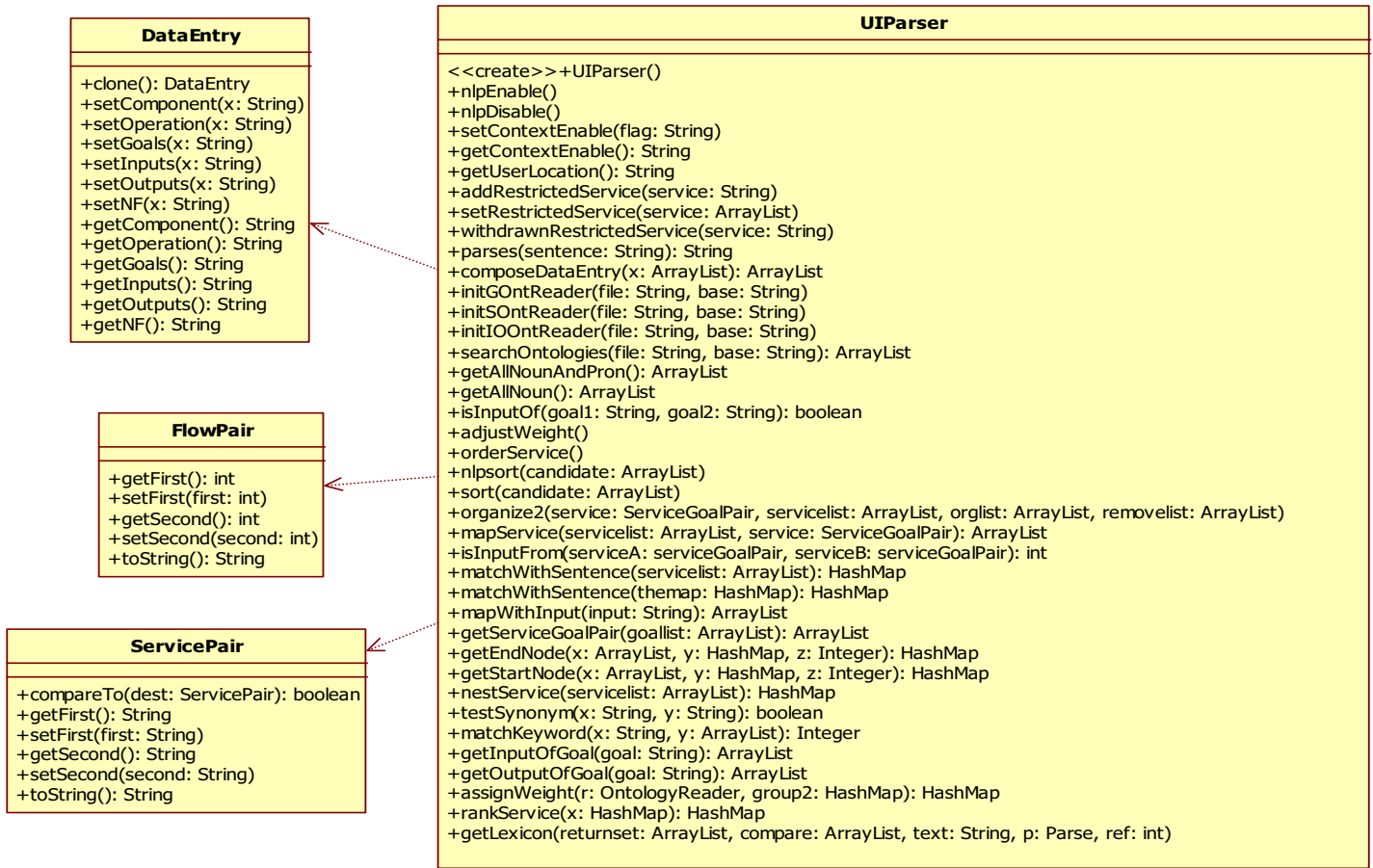
Figure 65: UML diagram of UIParser and dependent classes (3)
