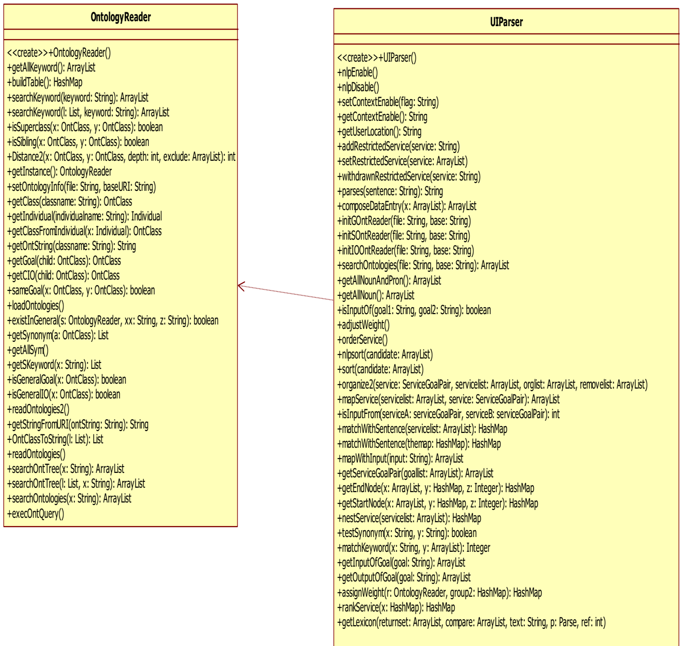
Figure 63: UML diagram of UIParser and dependent classes (1)
