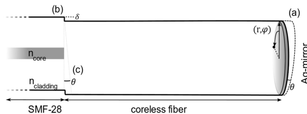
Figure 1. Schematic configuration of the challenges associated with the fabrication of fiberoptic interferometers based on core mismatch. The three parameters investigated are an end-face cleave angle (a), a lateral offset in the splice (b) and a tilted splice (c), as indicated in the figure.
