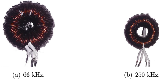
Figure 6.20: Switching at 66 kHz requires 2 \times stacked sendust core, CS358060, with 70-turns giving 565 \mu\text{H} , while at 250 kHz, only 1 \times stacked sendust core, CS330060, is sufficient leading to dramatic reduction in size of inductor.
