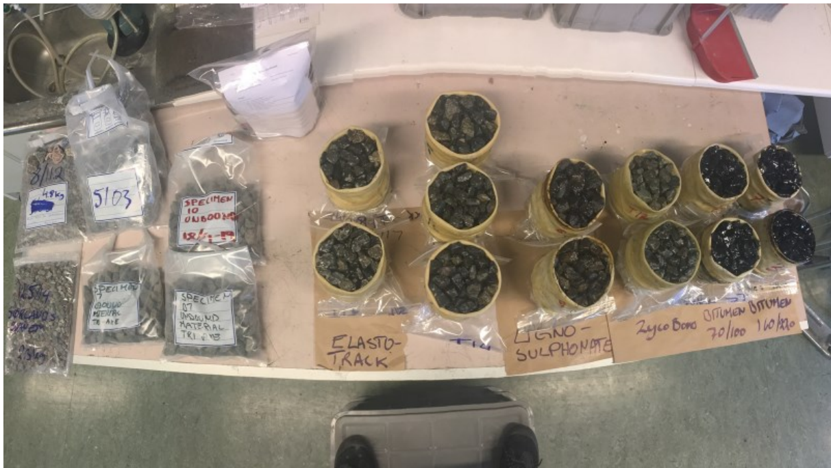
Figure 8: Tested samples. On the left side, aggregates tested without any additives. On the right side, stabilized samples.
