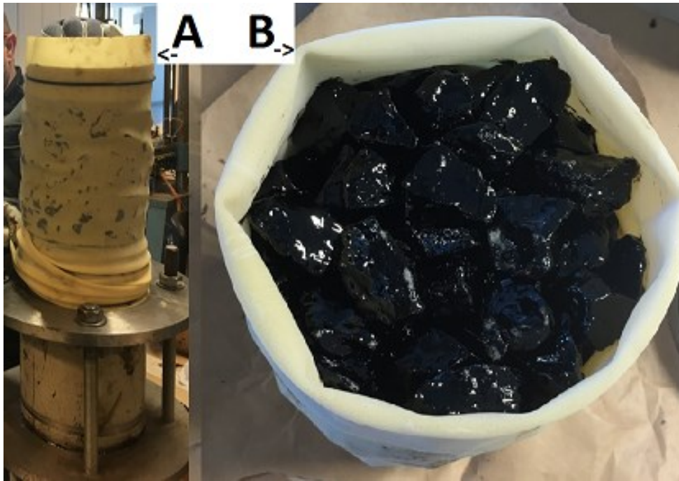
Figure 6: A) Taking the sample out of the mold, B) Sample is out of mold and placed for curing.
