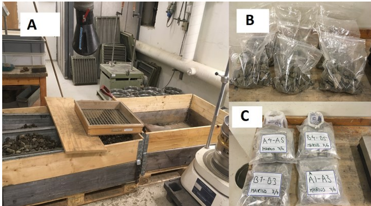
Figure 4: A) Hand sieving + machine sieving, B) Bags of 1.7kg with 70% 22.4/25 and 30% 25/31.5, C) Bags with complete sample rock material.
