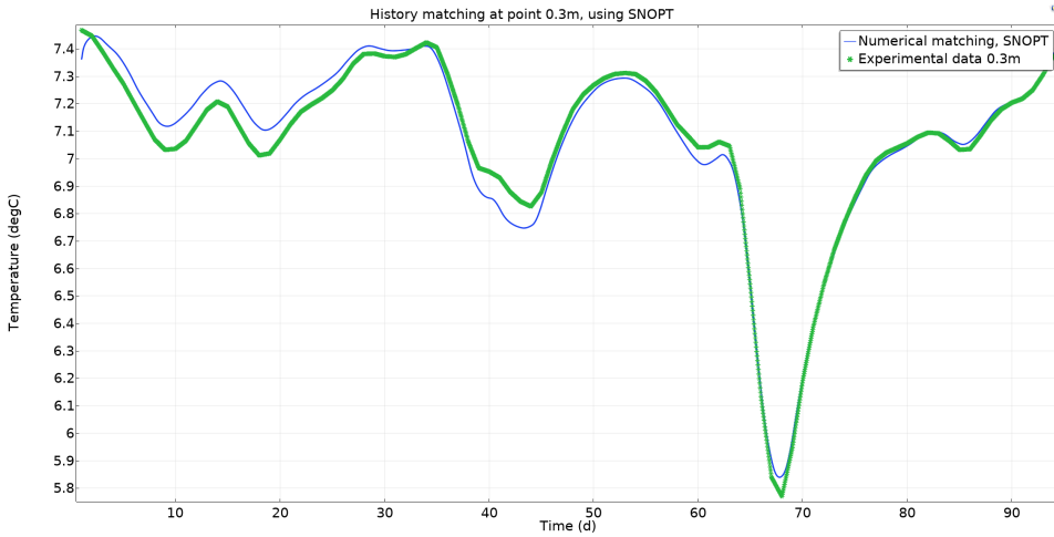
Figure 6.2: Result of the Parameter Estimation in measuring point 0.3m, study no.1, showing the reference data i.e. the measured temperature and the result from the numerical Parameter Estimation study.
