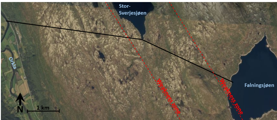
Figure 6.20: Black line illustrates the tunnel system and the red dotted lines represent possible weakness zones found in the tunnel.
