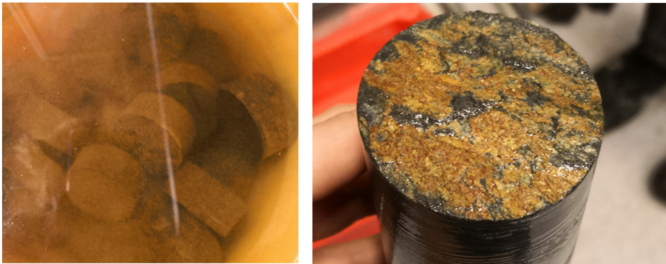
Figure 7.4: Red substance accumulated in water used to saturate the test samples(left). The same red substance was found on a weak plane which divided the rock cores during drilling.
