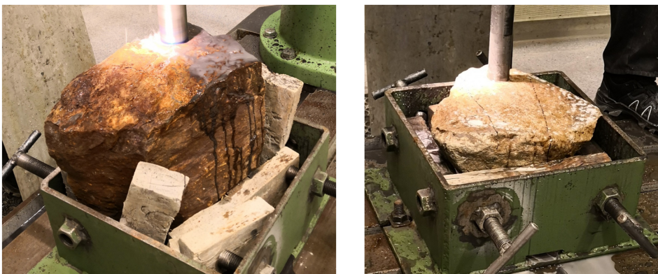
Figure 7.1: Rock core extraction from the quartzitic schist (left) and trondhjemite (right) samples.
