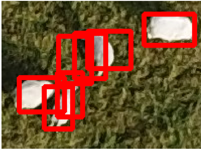
Figure 6.4: Example of overlapping bounding boxes in output. From DJI_0405.JPG with superclass at 832x832 pixels and a threshold of 0.1.
