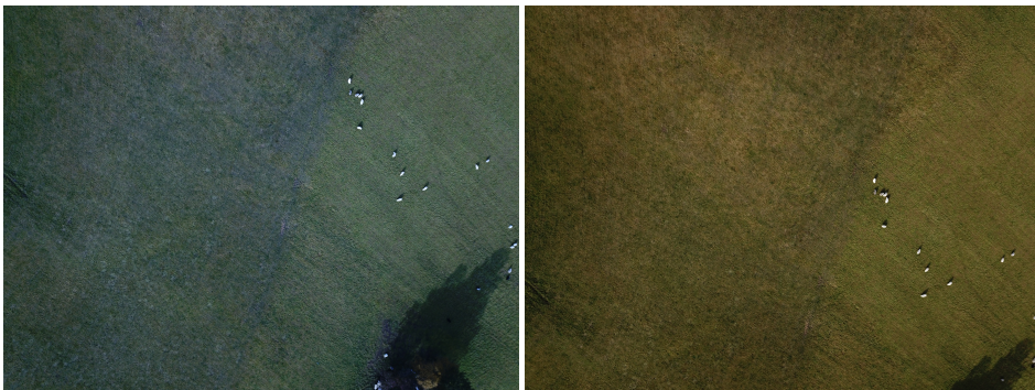
Figure 4.4: Example of exposure difference between images taken within 2 seconds of each other. DJI_0349.JPG and DJI_0350.JPG
