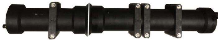
Figure 4-5 Illustration of the silhouette camera system within the high-pressure housing. Illustration taken from Davies et al. (2017).
