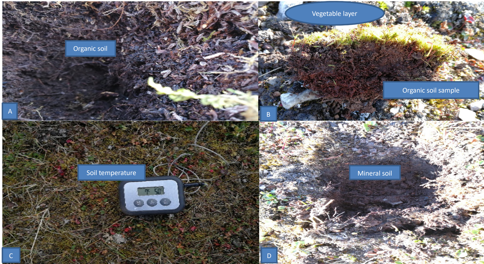
Figure 3.6: soil sampling: organic soil (A), organic soil samples with vegetable layer (B), soil temperature (C), mineral soil (D).
