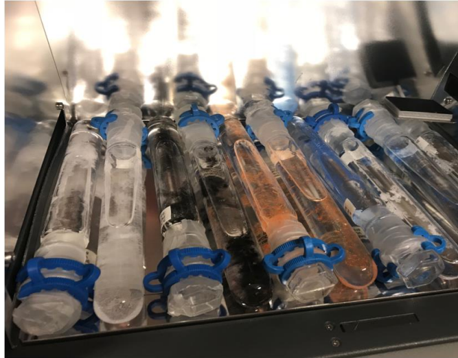
Figure 3.2. UV exposed MPFs in Atlas Suntest CPS+ chamber. (From left to right: PET (white) in SW, PET (white) in FW, PET (black) in SW, PET (black) in FW, PAN (orange) in SW, PAN (orange) in FW, PA in SW, PA in FW, PAN (blue) in SW and PAN (blue) FW.
