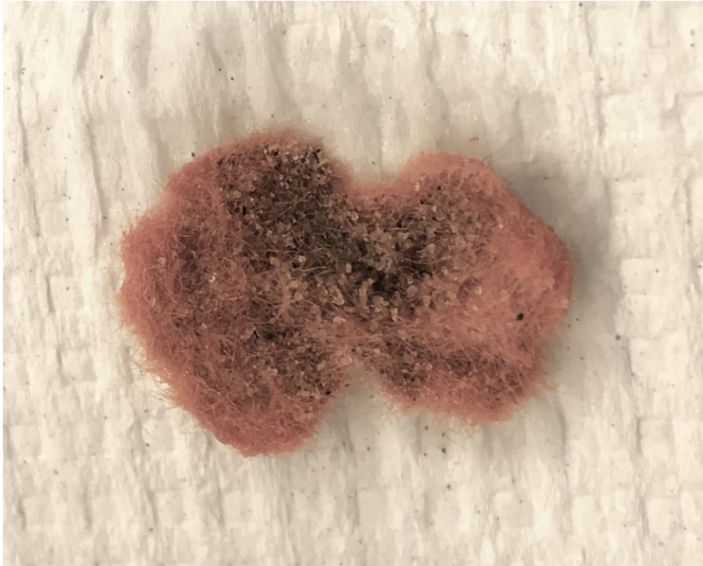
Figure 4.29. Separated orange PAN fibre cluster showing integration of sand particles
