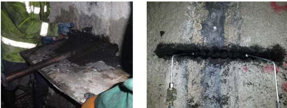
Figure 3. Installation of flatjack in the slot (left) and connection to the pressure measuring transducer (right).
