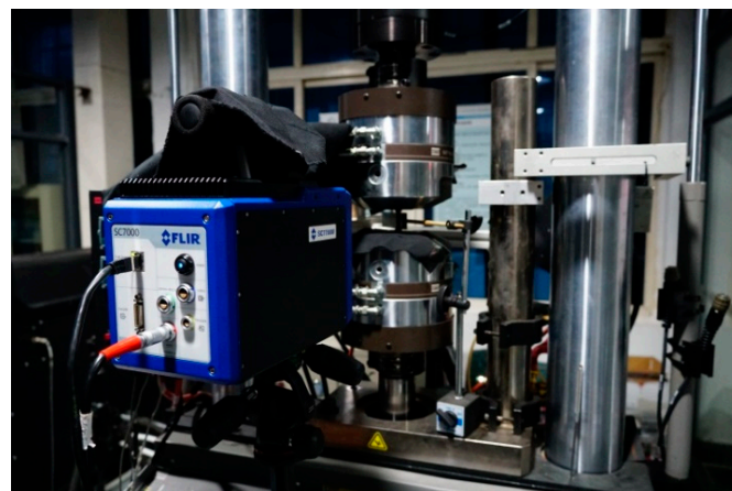
Figure 5. Installation diagram of the fatigue test and thermal measurement.
