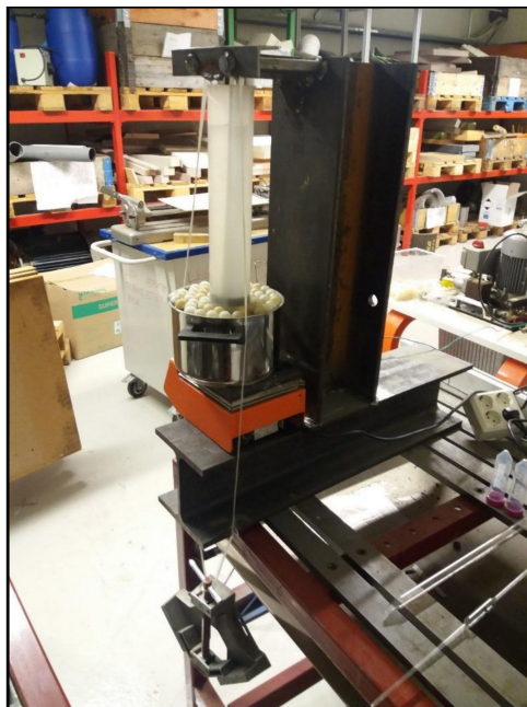
Figure 3. The glass fibre stress corrosion experimental setup.
