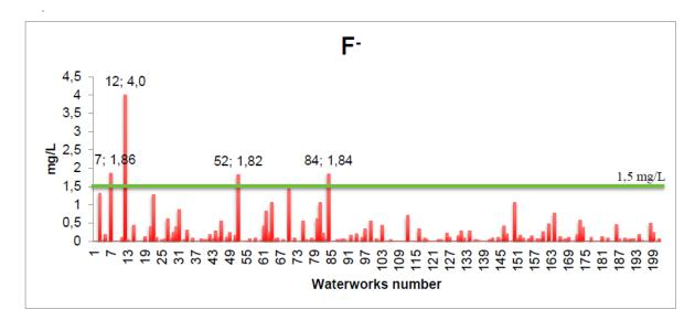
**Figure 3.1-1.** Analysed levels of fluoride (mg/L) in groundwater samples collected at 201 different waterworks in Norway in 2016. The green line indicates the Norwegian regulation upper limit of fluoride (1.5 mg/L) in water. Only one sample from each waterworks was available. Figure taken from Abiyos (2017).
