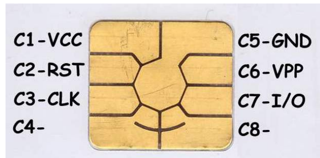
Figure 2: Smart Card Pin out 3
