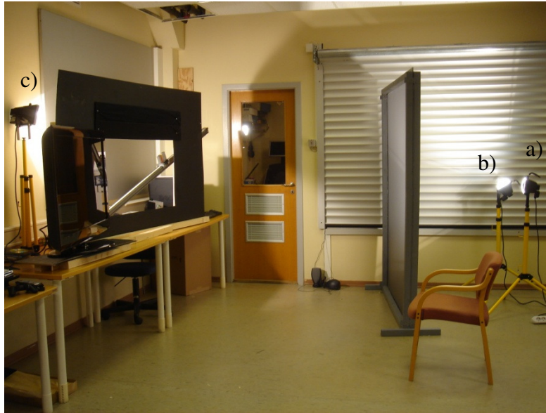
Figure 4-7: Light setup used during recording. a) key light, b) fill light and c) back light
