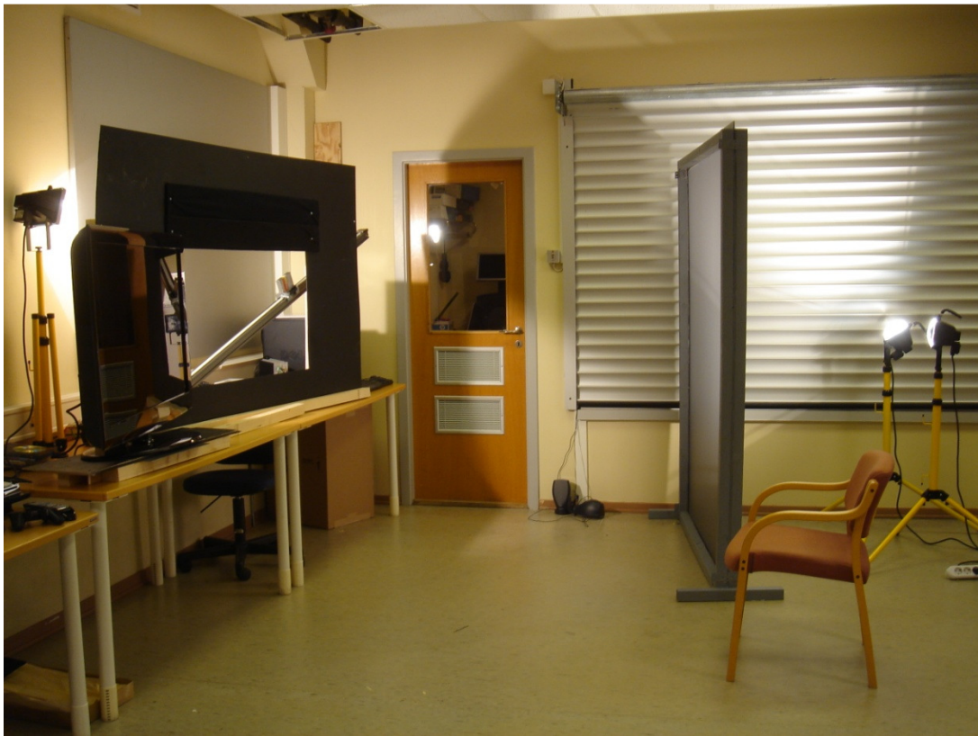
Figure 5-1: The placement of chair, screens, lights and model
