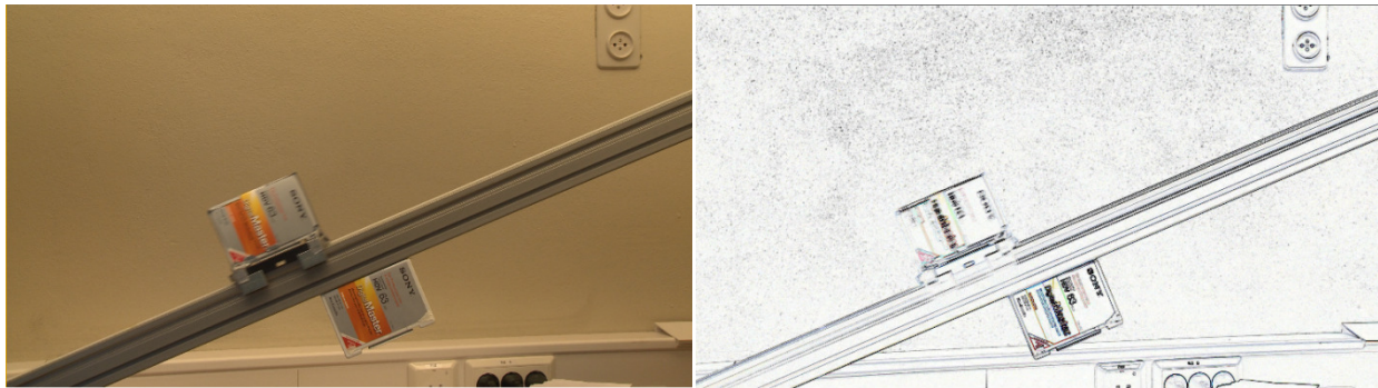
Figure 7-1: Scene with and without edge detection
