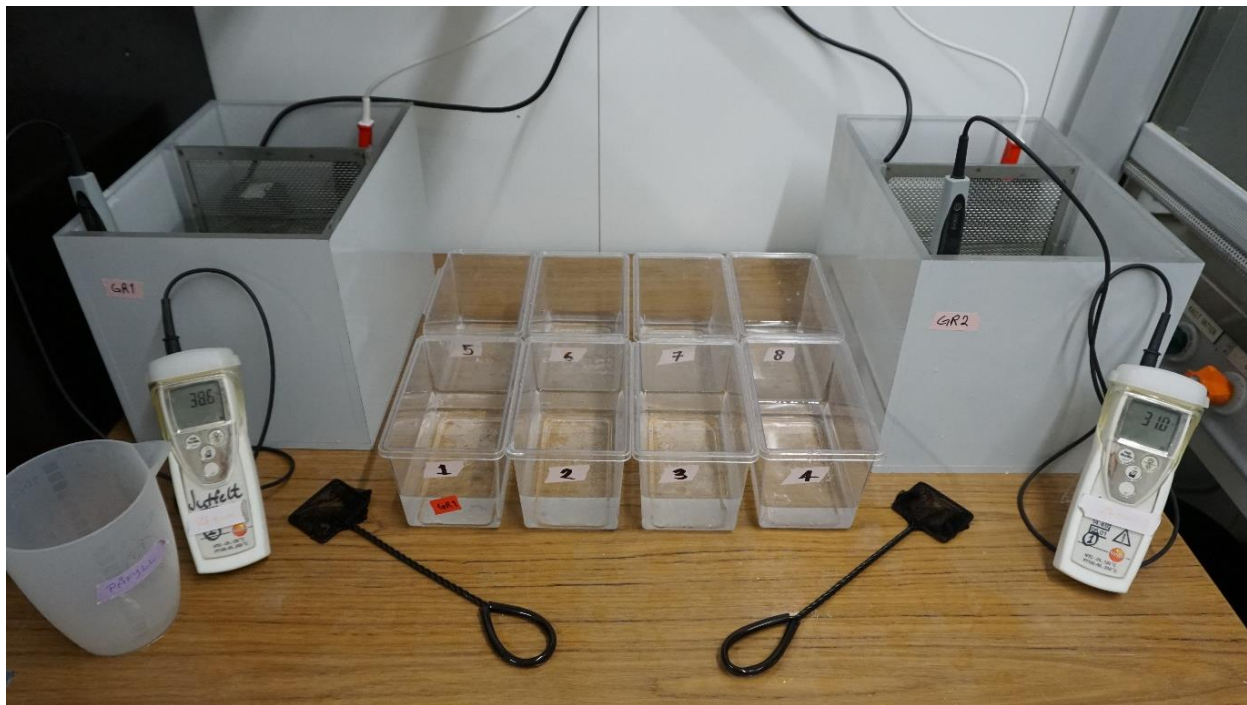
Figure 6. Experimental setup for testing CT_{max} , described in figure 5. Parallel trials with two setups for CT_{max} ; two set of numbered selection boxes (1 L) with ice water, nets, and thermometers and a water mug.
