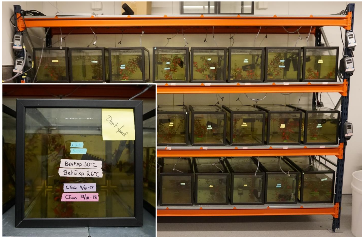
Figure 2. Tank setup in the acclimation room. Twelve of the tanks were used for our experimental fish; the six rightmost on the two upper shelves. Two filters in each tank and glass covers on top were adjusted to keep the water aerated and 28.0 \pm 0.5 °C. Close-up photo of the front of one tank with updated labels after each treatment or test.
