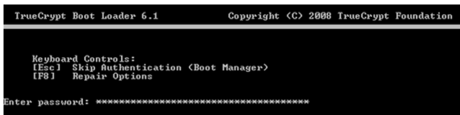
Figure A.8: As of TrueCrypt version 6.1, it is possible to turn off all text in the pre-boot authentication screen, preventing an adversary that is watching you start your computer from knowing that TrueCrypt is in use.
