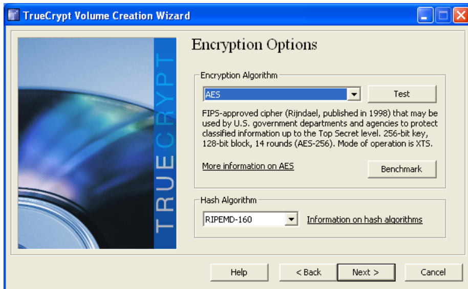
Figure A.3: TrueCrypt features strong 256-bit encryption using XTS mode with either AES, Twofish or Serpent block cipher, or all three of them in cascade mode.
