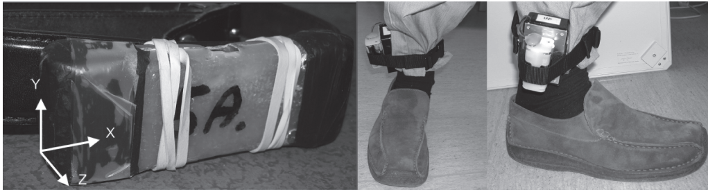
Figure 3.4: Wearable sensor equipment from earlier experiments. Left: Gait collector attached to a person's belt [29]. Right: Gait collector attached to a person's leg [43].
