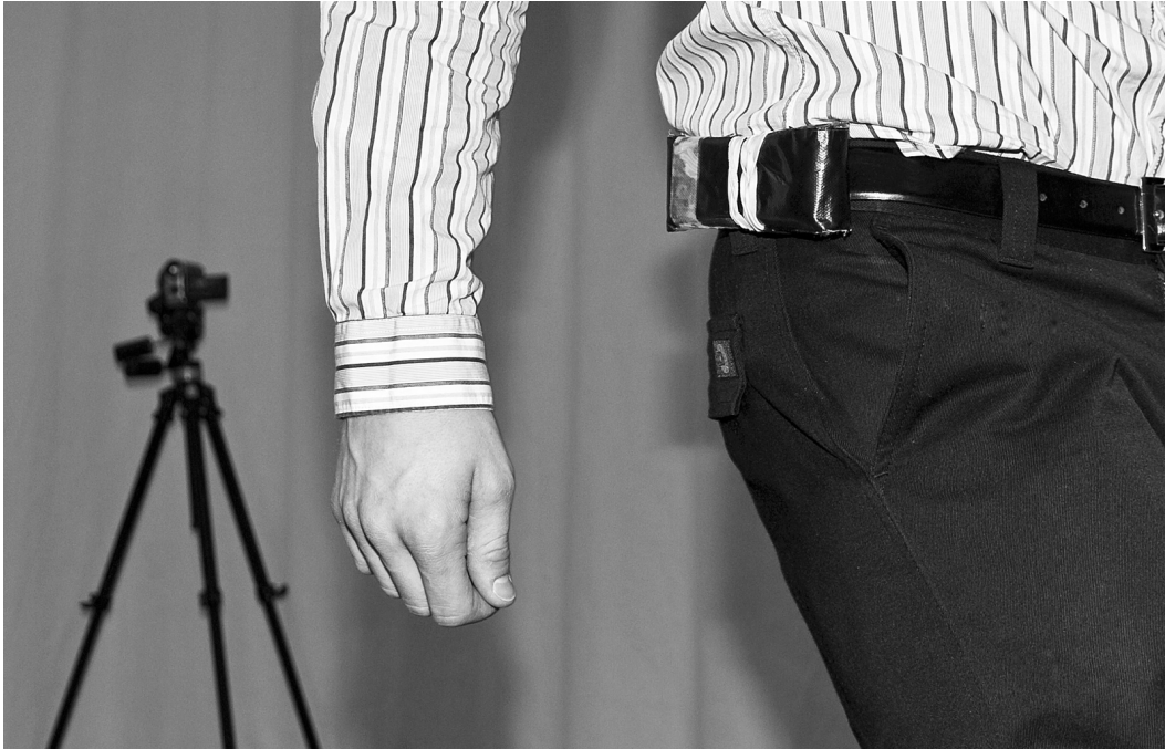
Figure 4.2: Gait collector attached to the hip, a video camera on a tripod in the back.
