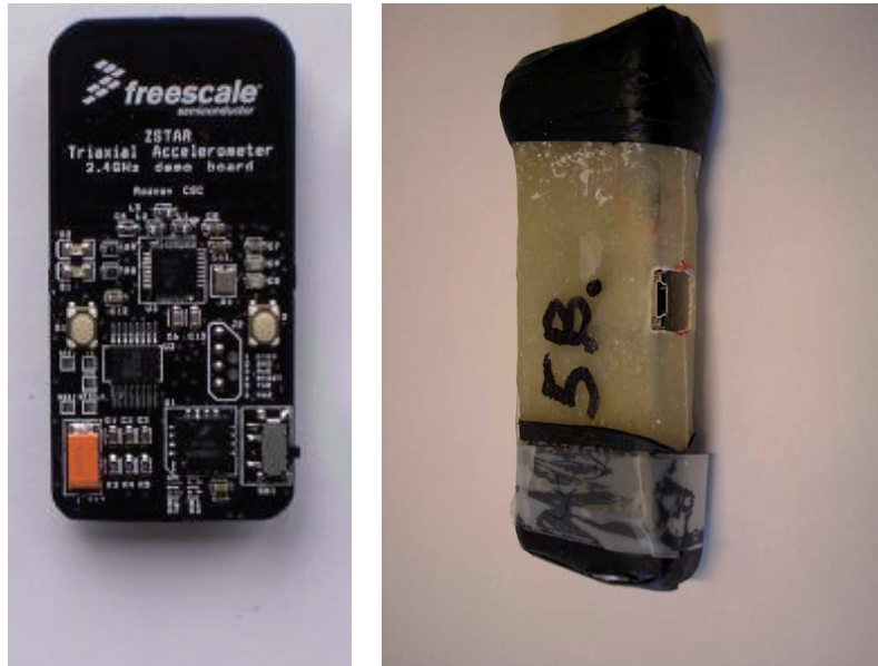
Figure 4.1: Available gait collection hardware. Left: The Freescale ZSTAR wireless accelerometer [53]. Right: The MR100 accelerometer [22].
