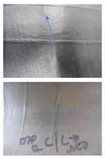
Fig. 7. (Upper) Inside of a XLPE power phase after 15,000 cycles at 1.1 %  $\Delta\epsilon$ ; (Lower) Inside of a XLPE power phase after 25,000 cycles. Arrow indicate axial object direction.
