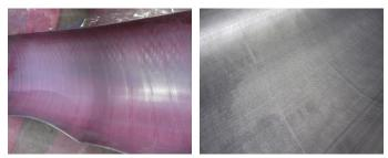
Fig. 10. (Upper Left) Inside of (run-out) MI power cable after 65,000 cycles at 1.02 %  $\Delta\epsilon$ ; (Upper Right) Outside of a (run- out) XLPE power phase after 40,000 cycles at 0.40 %  $\Delta\epsilon$ ;
