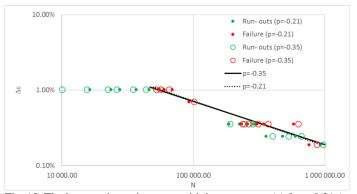
Fig. 13. The increase in strain rate sensitivity parameter (p) from 0.21 (as calculated from the small-scale experiments), to 0.35 determine a shift of the failure points below the calculated mean curve towards or above the curve. A higher strain rate sensitivity will in other words better explain the observations.
