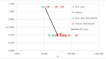
Fig. 6. Full scale results for XLPE power phases together with the results normalized to the average testing strain rate and calculated the maximum likelihood function.
